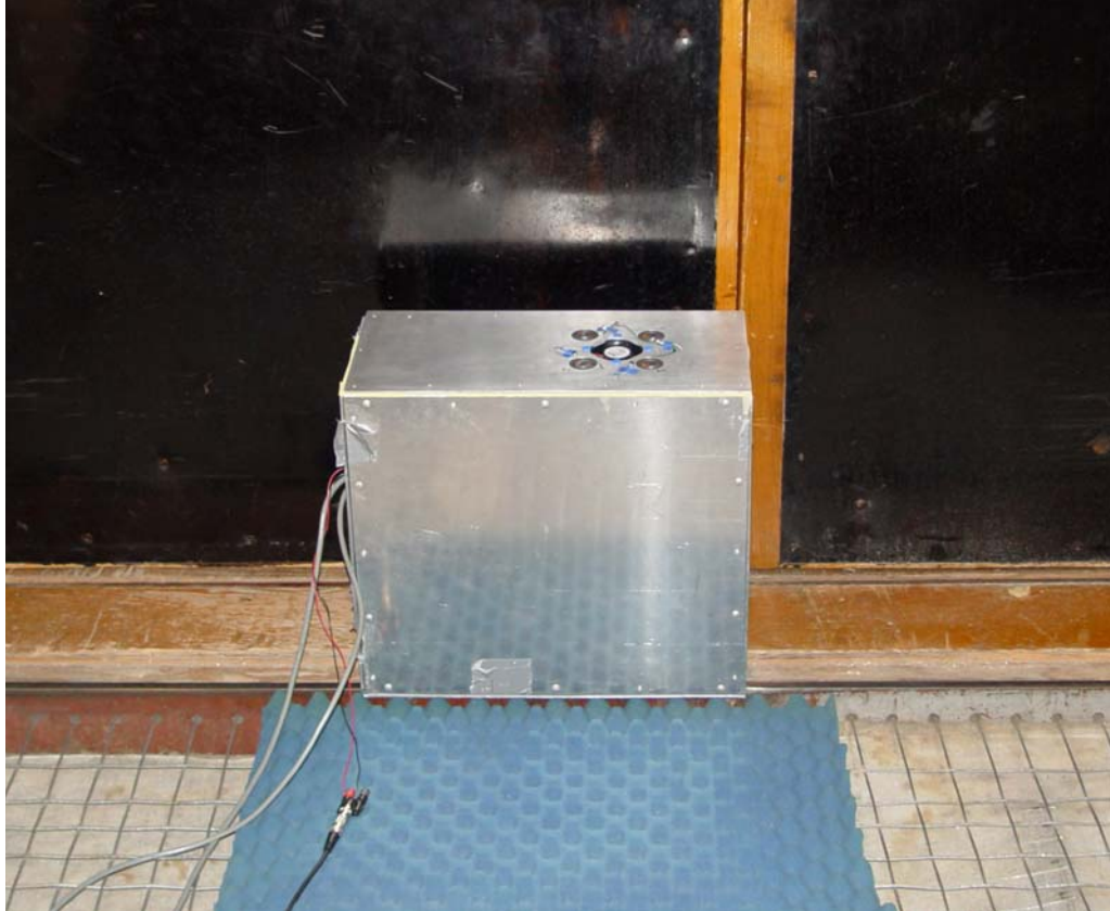
Figure 5.8 Mock computer case with fan and ANC system relocated to rigid wall within the anechoic chamber.
