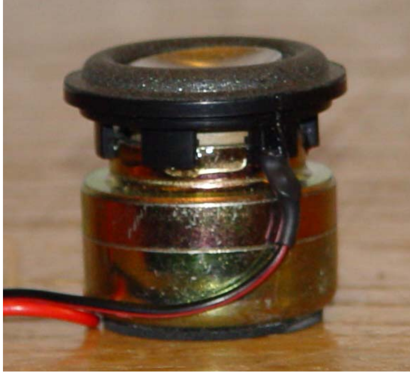
Figure 4.2 1” Loudspeaker used as secondary source for ANC.
